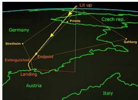
3D triangulation of the atmospheric trajectory of Neuschwanstein by the European Fireball Network stations.
