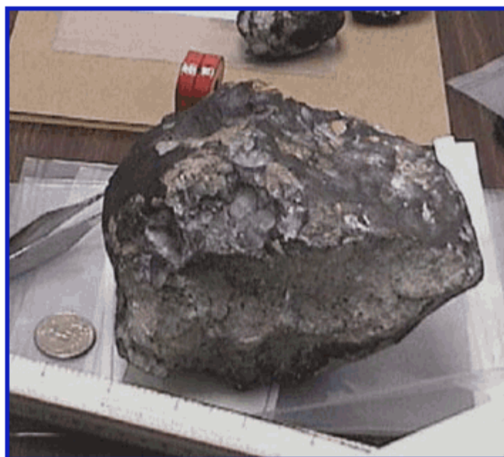
The 2.5-kilogram meteorite fragment that caused the damage. It displays a typical black fusion crust, which is broken in places revealing the lighter-colored interior.
